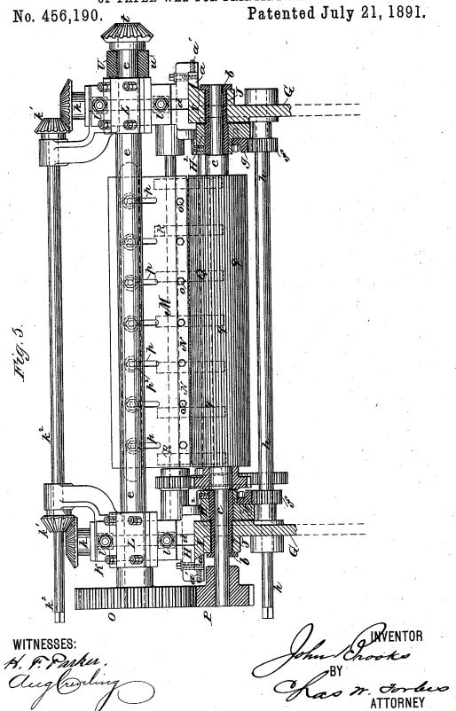
MECHANISM FOR CUTTING OR PERFORATING VARIABLE LENGTHS OF PAPER WEB FOR PRINTING PRESSES.
