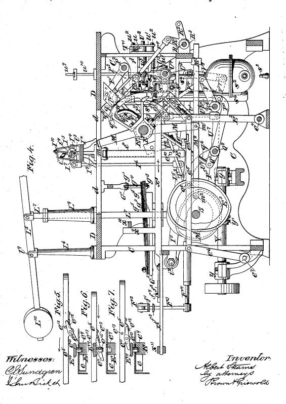
MACHINERY FOR SECURING WRAPPERS OR LABELS AROUND BOXES, CAKES, &c.
