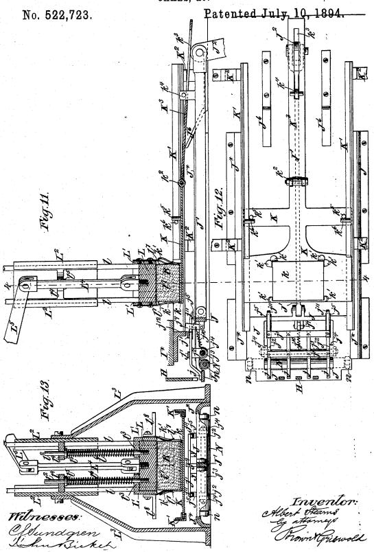
MACHINERY FOR SECURING WRAPPERS OR LABELS AROUND BOXES, CAKES, &c.
