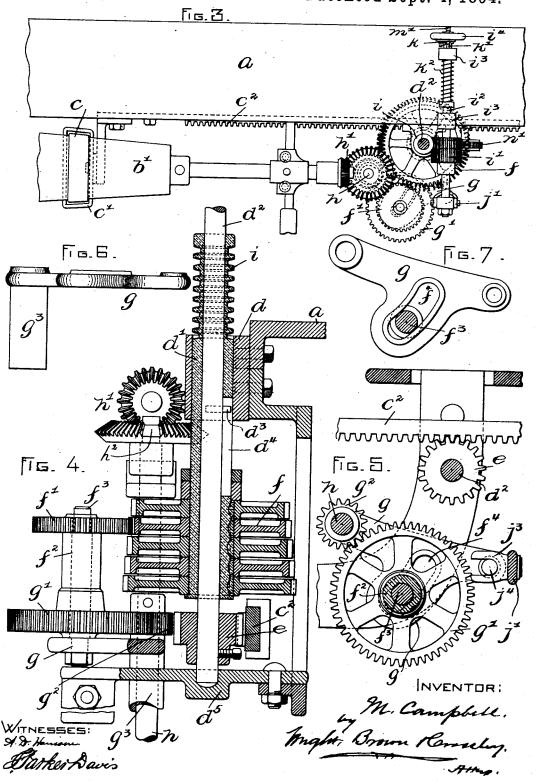
ADJUSTING MEANS FOR BELT SHIFTING MECHANISM OF ROVING FRAMES.
