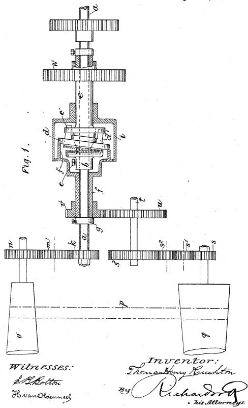
GEARING FOR IMPARTING DIFFERENTIAL MOTION IN MACHINERY. No. 526,413. Patented Sept. 25, 1894.
