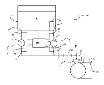
casting apparatus for the production of a sheet of material containing alkaloids.
